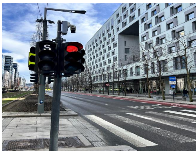
Figure 29 Actinode camera on top of traffic light for data collecting at DEG
