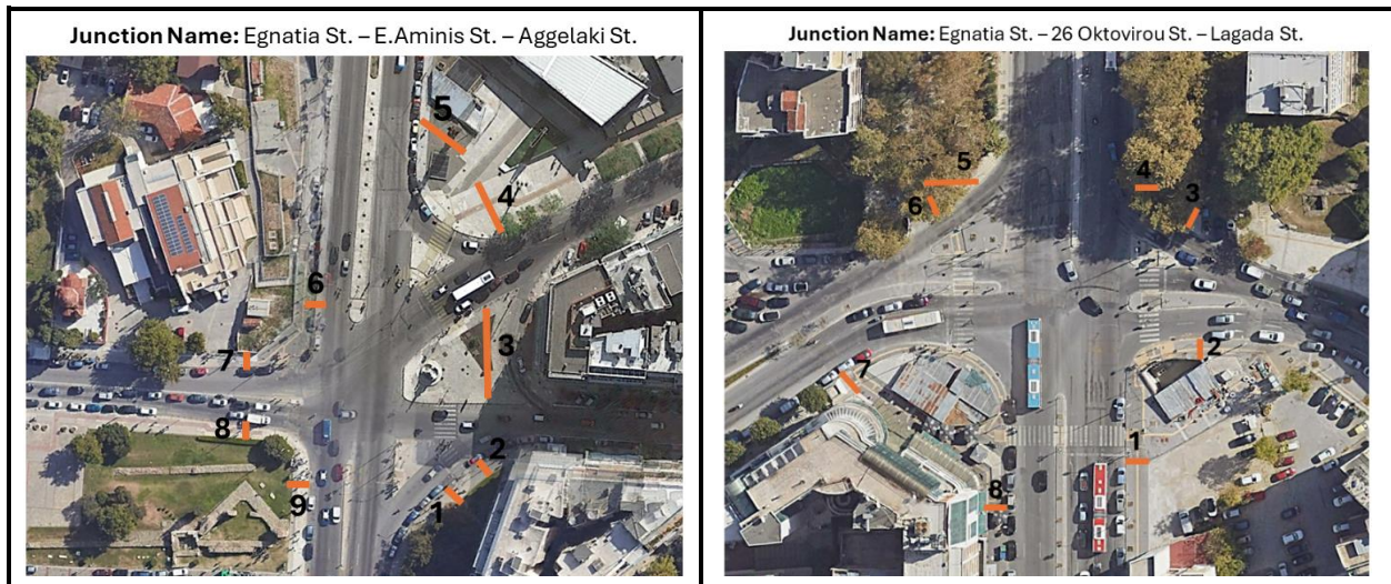
Figure 3 Locations of pedestrian flow measurements at two major signalized junctions on Egnatia St.
