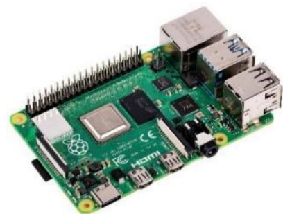
Fig 30. Raspberry PI model 4 selected to process the multimodal panel information
